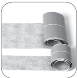
Use the Edge Sealing Tape (provided in Kits) to seal both ends of the Heating Film. The Edge Sealing Tape comes in two different widths (4.8" wide and 2.4" wide). The 4.8" wide tape is designed to seal the edge of the sheet to which the Harness or Adder is attached. The 2.4" wide tape is to seal the edge of the sheet that does not have a Harness or Adder attached, or any section of the Heating Film that has been cut as part of the installation process. Simply
