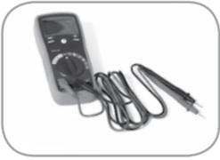
A DIGITAL multi-meter is required to perform the resistance test. Analog meters (which have a needle rather than digital readout) are not recommended, as they do not provide accurate enough reading when calculating the formulas.
